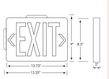
NSi's die-cast aluminum LED exit lights have fully automatic operation at 120 or 277 VAC, in AC only or battery units. Die-cast LED exit lights have a universal mounting canopy for side or top installation. Excellent energy savings of LED in a curved design with universal K/O chevrons. Face plate is brushed aluminum.
