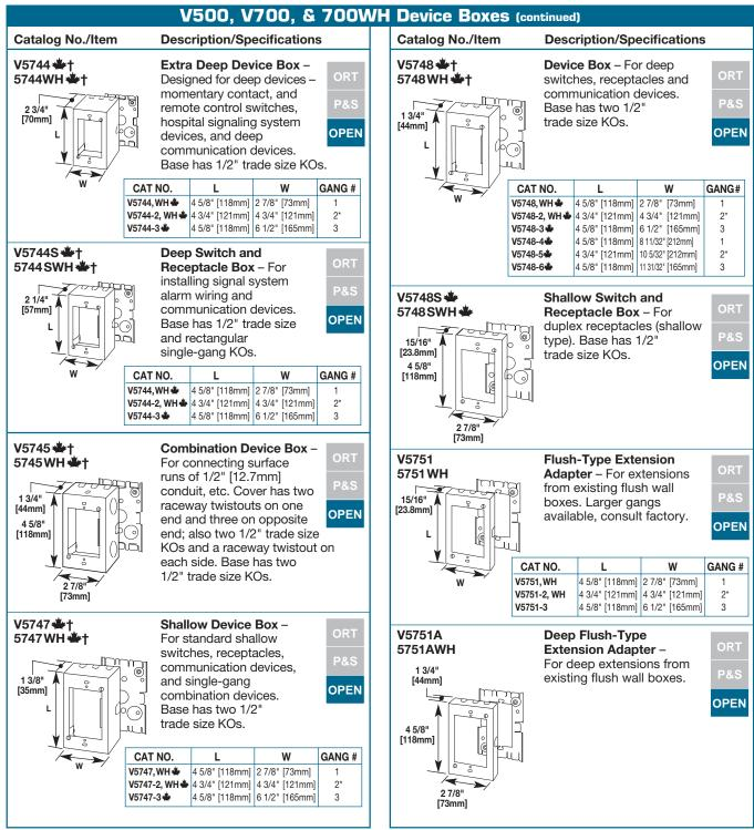
**NOTES:** Covers on this page have double twistouts. Break out lower twistout for use with V500, and both twistouts for use with V700. \* V5744-2 and V5744S-2 Base and V5747-2 and V5748-2 Base have 1/2" and 1" concentric trade size KOs and a 1 13/16" x 2 7/8" [47mm x 73mm] rectangular KO to permit mounting on a one-gang in-wall outlet box.
